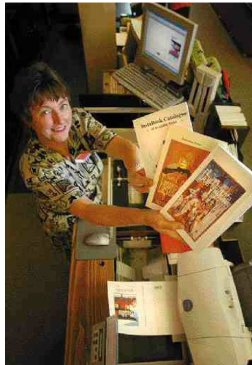
Anne Laird of Book Express uses the InstaBook, which allows a customer to print, bind and cover a copy of a book that may be out of print. It can also be used by those who want to self-publish.
